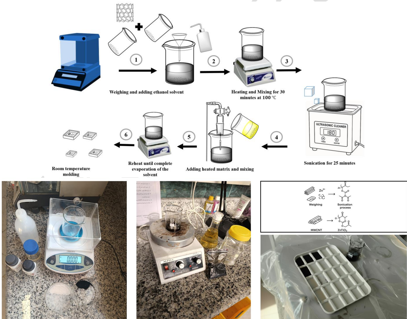
Fig. 4. Experimental procedure for laboratory-scale nanocomposite fabrication
