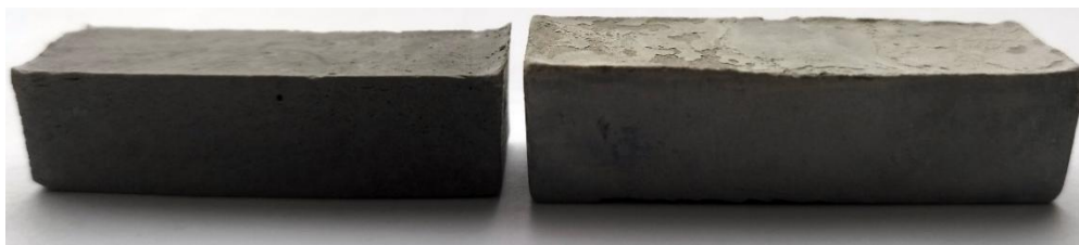
Fig. 5. Visual appearance of GS 20 F 0.5 (left) and PS 20 F 0.5 (right) composites
