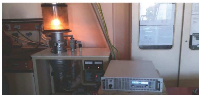
Fig. 1. Working evaporation chamber
