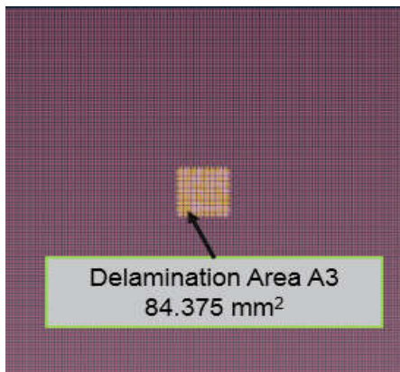
Fig. 3. Top view of delamination incorporated.
